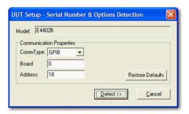
NOTE: Be sure that the DUT has been connect to the GPIB cable and is turned on. This function will automatically find the DUT and query it for serial number and installed options.
