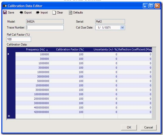
The initial values will be set to their defaults. The table is similar in operation to an MS Excel spreadsheet. Enter the correct values as indicated by the column headings. To insert a new frequency point scroll to the bottom enter the new data. The table will automatically sort when you have finished with the new row. Enter the appropriate trace number and then select the next calibration due date.
